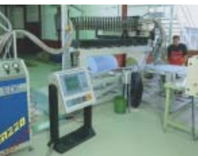
Special CNC machine to apply the sealing compound
